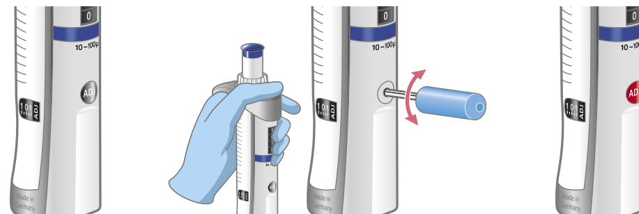
Figure: Adjustment of an air-cushion pipette und clear visible identification (sticker).
