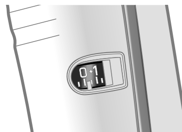
Figure: Adjustment window of an air-cushion pipette
